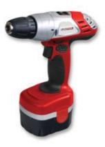
Drill Combi 18V, 2 x Batteries, UK Supply Voltage AC: 230V Chuck Size: 10mm Battery Capacity: 1.2Ah Battery Type: NiCd Battery Voltage: 18V Chuck Size: 10mm Chuck Type: Keyless Max Torque: 11.5N-m No Load Speed: 3500rpm No. of Batteries: 2 No. of Speeds: 2 Steel Drilling Capacity: 10mm **Torque Settings: 16** Weight: 1.6kg Wood Drilling Capacity: 13mm
