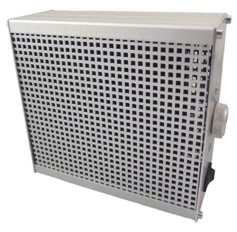
A well proven unit, with robust aluminum-casing and pierced frontplate, that cannot be inadvertently damaged by hot solder tips. The absorber can be used either as a table appliance or higher up with a tripod, to be ordered seperately (with round base), with variable inclination angle. Power requirement: 220/240V/18W, air throughput: 170m³/h, noise level: 40dBA, housing: anodized aluminum, dimensions: 150x140x55mm
