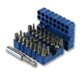
A 33 piece security bit set ideal for use with cordless screwdrivers & drills. Compact pocket sized bit box. Supplied with 1 x 60mm bit box. Torque bits: T8, T10, T15, T20, T25, T27, T30, T35, T40 Hex bits: 2, 2.5, 3, 4, 5, 6mm Tri-Ling bits: #1, #2, #3, #4 Spanner bits: #4, #6, #8, #10 Cross-head bits: #6, #8, #10 Magnetic bit holder.
