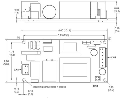
Mounting holes marked with  $\begin{center}$  must be connected to safety earth
