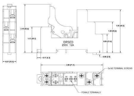
Tolerances: ± 0.02 in / 0.5 mm. All dimensions are in: inches [millimeters]
