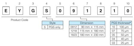
\* PGS thickness of 17 μm, 10 μm does not support as single item.
