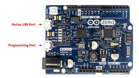
Either USB port can be used for programming the board, although using the Programming port is recommended due to the way the erasing of the chip is handled:
