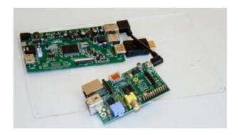
Using the M3 bolts to secure the Pi in place (the first revision of Raspberry Pi's do not have mounting holes, if you are using one of these skip this step). Push the bolts through the driver board and then through the Raspberry Pi's mounting holes. Sometimes this can be a bit tight. Follow up by adding the nuts to secure the Pi to the driver layer.
