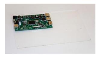
Plug in the HDMI connector to the driver board.
