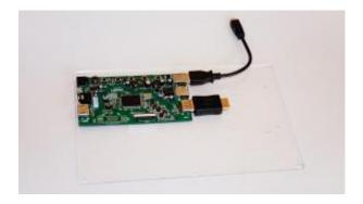
Next step is to add the Raspberry Pi, firstly plug the micro USB connector in to the Pi, followed by pushing the Raspberry Pi to plug in to the other side of the HDMI
