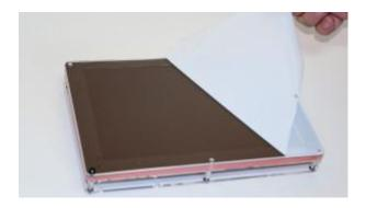
Add the remaining 4 bolts, bear in mind pushing a bolt through the 4 layers will be a bit tight. Add the hex spacer to the back using finger tightness, do not use any mechanical tool to tighten the spacer as it could lead to cracking of the layers and potentially damage the LCD panel.
