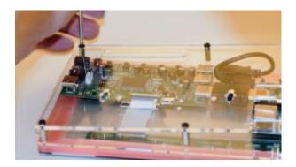
All that is needed to finish is stick on the acrylic buttons. Each button has peel-able backing so the button can be stuck straight on to the tactile buttons of the driver board if you wish.
