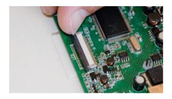
To insert a new or reseat a ribbon cable, slide the ribbon cable in to the connector, ensuring the grip is pushed out, firmly insert the cable with the contacts facing down and blue tape upwards. Push the grip back in to the connector to lock the cable in place.
