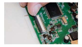
Insert the ribbon cable in to the connector, and push the tab back in place to grip on to the ribbon cable. The ribbon should be straight, and the tab firmly in place.
