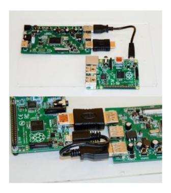
Using the M3 bolts to secure the Pi in place, push the bolts through the driver board and then through the Raspberry Pi's mounting holes. Sometimes this can be a bit tight. Follow up by adding the nuts to secure the Pi to the driver layer.
