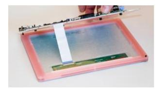
Fix everything together by screwing on the hex spacers on to the 2 bolts, don't use any mechanical tools to tighten the spacer, as this could lead to damage with the acrylic layers and LCD panel.
