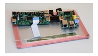
The connector works by gripping on to the ribbon cable with the black tab to hold it in place, in much the same way as the Raspberry Pis' camera connector does. Using thumbnails, carefully push the connector away from the driver board;
