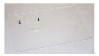
Do the same again for the other hole, followed by another M2.5 nut. Push the driver board on to the screws, with the LCD connector next to the cutout. Screw the remaining 2x M2.5 nuts on top of the driver board to secure it in place. If it is too fiddly to grip use a pair of pliers to grip the nut whilst screwing it in place.
