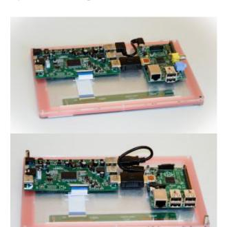
Now you can turn over the unit to add the remaining bolts and hexagonal spacers. Peel around the edge of the first layer to uncover the remaining screw holes – Or remove the protective layer completely if you are feeling confident!
