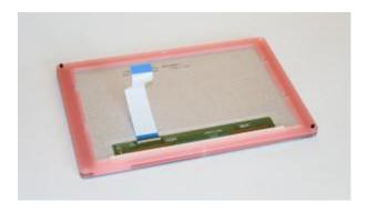
Add the layer 3 on top of the unit, pay attention to the notches in sides, these are there to give some room for the driver board screws so no damage is done to the back of the LCD panel.
