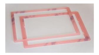
As you will also see, one of the sides is thicker than the other. The reason for this is on the LCD panel itself, one side of the metal is thicker, so the design is to overcome this and also keep the screen central to the unit.
