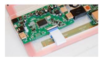
Carefully lift up the driver layer to pull the slack of the ribbon cable through the cut out, and place it back down on top of the unit, making sure the screws feed through the holes in the driver layer.
