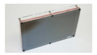
If you haven't already tried the LCD screen in the test above, all that is needed now is to rip the front protection layer off – If you haven't done already – Add a mouse and keyboard, and a 5.2V or 12V power supply.
