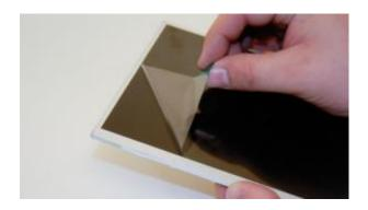
The LCD panel should fit snugly within layer 2. Carefully pick up the unit to double check everything is placed the right way around. You shouldn't see the metal of the LCD panel (providing the black HDMIPi layer is used).
