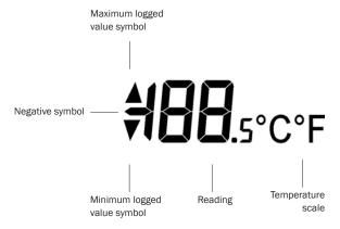
The LCD shows three different recorded readings, which can be cycled through using the built-in push button. The most recent logged temperature, maximum logged temperature and minimum logged temperature can be displayed. In addition, logging and alarm status is shown using two high intensity LEDs.
