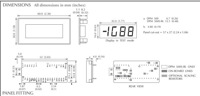
Fit the bezel to the front of the panel and locate the meter into the bezel from behind. Alternatively the meter and bezel may be assembled before fitting to the front of the panel but care must be taken not to use excessive force. Finally fit the window into the front of the bezel.
