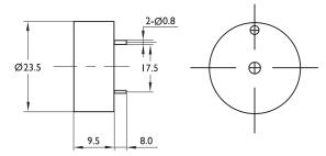
Dimensions: Millimetres Tolerance: ±0.5mm
