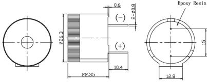
Dimensions : Millimetres Tolerance: ±0.5mm
