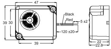
Dimensions: Millimetres Tolerance: ±0.5mm
