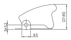
Dimensions: Millimetres Tolerance: ±0.1mm
