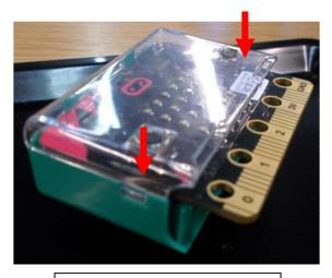
Then secure the cover by pushing down on either side.
