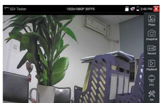
IPC tester's HDMI output port can be use as SDI to HDMI converter to output HD SDI image to HD TV monitor. Select relative functions on the right side Toolbar to operate, "Snapshot", "Record", "Photos", "Video playback", "PTZ control", "Video Brightness and Storage set".
