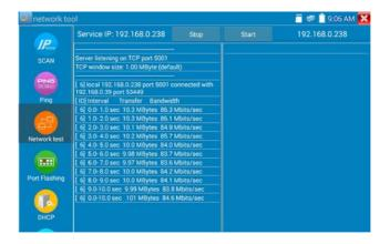
b). Start send packet test: Using the second IP tester, type in the Server's IP address at the top right corner of the screen. This app is used to send packets for network speed testing. Click the "Start" button to send the packets and start testing.
