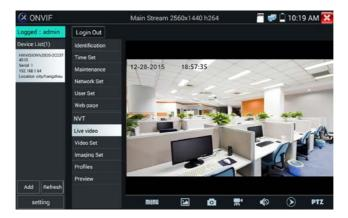
ONVIF PTZ control: Tap the image in the direction you want the PTZ camera to move. For example, tap the left side of the image to move left, right side to go right, up to go up, and down to go down.
