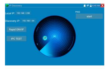
Local IP: Tester's IP address where the tester can auto-modify the tester's IP to the same network segment with the scanned camera's IP
