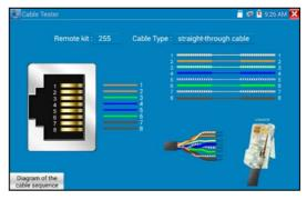
Test LAN cable or telephone cable.
