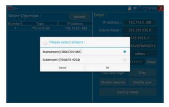
If the camera does not support non-verification login, select "camera" from online detection menu, and input correct user name and password, then click "log in". After logging successful, you can test it.
