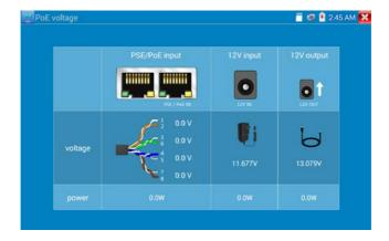
Warning: Do not connect a device with input power over 17V to the tester's "12V IN" port, otherwise it will damage the tester.
