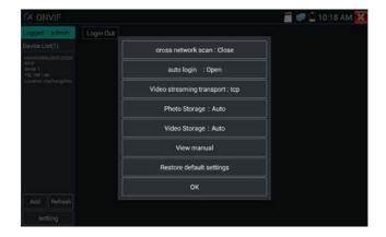
Cross network scan: After opening this function, enter "Settings," "IP Settings" and "Advanced" to add other network segments IP so "Rapid ONVIF" function can cross network segments to scan camera's IP.
