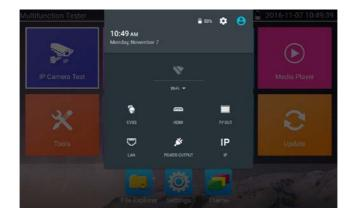
**HDMI:** Click HDMI to enter the HDMI input mode, where the tester can display a dual test window (picture in picture) with IP & HDMI inputs or Analog & HDMI inputs.
