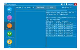
Or use tester as a Server and the computer as test Client (select Client, input tester's IP address to test)
