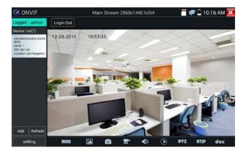
While in the live video, the Video Menu is across the bottom of the screen and provides access to the following tools: Snapshot, Record, Photo, Playback, PTZ, RTSP and docs.
