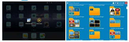
The Media player can browse video and image files. It supports the video formats of MP4, H.264, MPEG4, and MKV. The IP tester's recorded files can play directly via the Media player. The Media player will automatically display the video files from the SD card. Click on the desired file to play. Click RETURN to exit.
