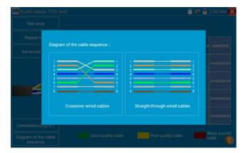
For reference only: A straight-through and cross-over cable diagram
