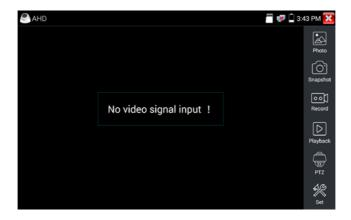
With an AHD signal input, the tester will display the image resolution on the top bar. Double tap on the screen to make the image displayed full screen.
