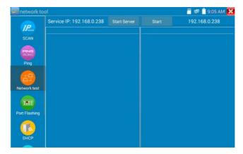
a). Start the server: Click "Start Server" button to use the first tester as a Server. It will display its IP address at the top of the screen.
