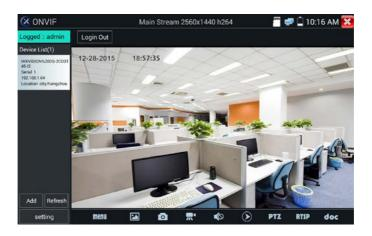
The tester lists cameras name and IP address on the left of screen. Tester can auto login camera and display camera image. Factory default use admin password to auto login, if you modified the password, then default use the modified password to log in.
