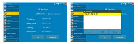
After setting an advanced IP address (refer to the photos above), the unit can test two network segments (192.168.5.0) and (192.168.1.0) at once.
