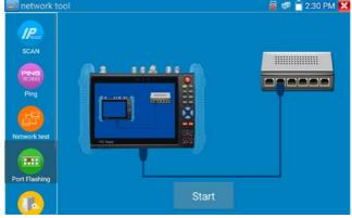
If the tester and PoE switch are connected correctly, the LAN port of the POE switch will flash at a special frequency, if not connected correctly, no any changes will occur on the LAN port.
