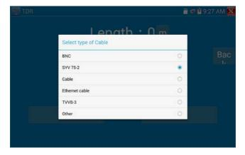
3. Click "+"or "-" to adjust wave speed, while display length is the same as the actual Length. Click "Save" to save calibration data and then it can be used for the same cable testing next time.
