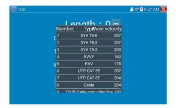
**User-defined calibration**: Choose the cable 100 meters to 200 meters (more than 50 meters); click "Cable" and "Type" to select user-defined 1 for calibration. Eleven groups can be set.
