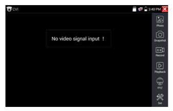
With HD CVI signal input, the tester will display the image resolution on the top bar. Double-tap on the screen to make the image displayed full screen. The tester supports resolution as follows  $1280x720P\ 25FPS\ /\ 1280x720P\ 30FPS\ /\ 1280x720P\ 50FPS\ /\ 1280x720P\ 60FPS\ /\ 1920x1080P\ 25FPS$   $1920x1080P\ 30FPS$
