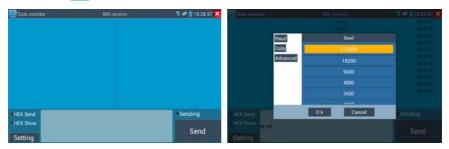
Click "Setting" to choose the baud rate of RS485; it must be the same as the DVR or the Control keyboard. The DVR or Control keyboard will send the code to the tester, if it can be read, the protocol will show on the upper right, such as PelcoD.
