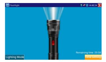
While in the flashlight app, click the red button on the flashlight to turn on the LED lamp. Press it again to turn it off. If you don't press the red button to shut off the lamp and press the button to exit the app, the lamp will stay on. Click the Time Setting button to set a timer that will shut off the lamp.
