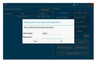
Factory reset: camera will be soft reset and the device's user name, password and network settings will be saved; other settings information will return to factory reset values.
