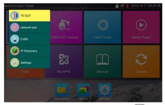
Press the MENU key to turn it on, arrow keys to switch functions, and ( to enter app; tap outside the menu to exit.
