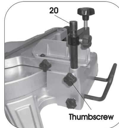
The work-piece clamp (20) can be fitted to either side of the saw blade depending on the work-piece size and the type of cut being performed.
