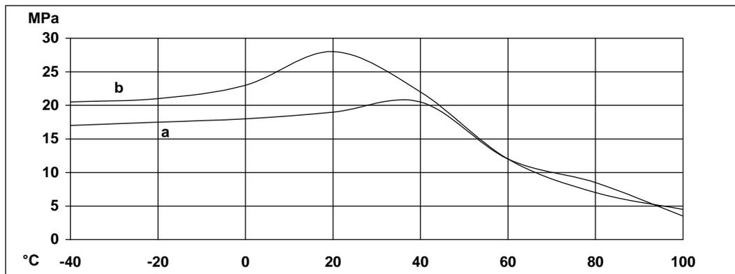
**Roller peel test (ISO 4578)** Cured 16 hours/40°C
