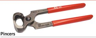
Optimised jaw design for effective gripping & extracting of screws, nails, fixings, etc. Specially profiled cutting blades for cutting metal rod & wire. High alloy steel, drop forged, hardened & tempered for exceptional strength & durability.
