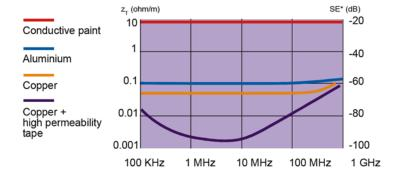
\*SE = Shielding efficiency : equivalent to a  $50\Omega$  load.
