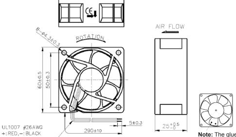
Note: The glues on the impeller is for impeller balance. Do not remove it.
