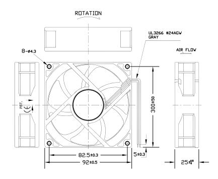
1.Air Flow Direction: Toward Label side.2.Best Mounting Direction: Any orientation.
