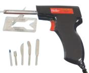
When the Therma-Boost mode is activated, the high-performance 30W/130W/230V soldering gun reaches its maximum temperature in less then 45 seconds. In standard operating mode, it operates with an output of 30 watts. It is ideal for cutting or processing synthetic materials, foams and styrofoam, as well as for soldering. When the Therma-Boost switch is pressed, the red lamp lights up and an output of 130 watts makes a quick burst of heat available.
