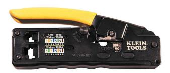
The Compact Ratcheting Modular Crimper/Stripper/Cutter provides fast, reliable connector termination for voice and data applications. This all-inone tool, cuts, strips, and crimps CAT6, CAT5, CAT3 and flat-satin voice cables. Its direct lateral crimp action provides more even, precise contact termination across all pins than ordinary indirect crimping tools. A compact, ergonomic design provides easy usage and storage.
