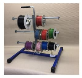
Constructed from mild steel with a painted base and plated top, The tree can hold several rolls of wire in various sizes. As the branches have no pins or clips to retain rolls changing rolls is made quick and simple. Ideally suited for use on benches and can be carried using top handle for moving around the workshop and storing away
