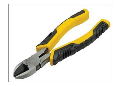
The Stanley Tools ControlGrip™ Diagonal Cutting Pliers are made from forged carbon steel with an induction hardened blade and tempered jaws for long life. Precision milled cutting edges and pivot for smooth opening and closing of the jaws.
