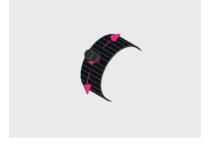
To adjust focus, hold the camera with the lens facing away from you. Turn the focus ring, labelled 'NEAR ◀▶ FAR', anti-clockwise to focus on a nearby object. Turn it clockwise to focus on a distant object. You may find you need to adjust the aperture again after this.
