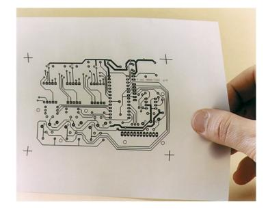
A specially formulated translucent film for the production of high resolution PCB artworks directly from any laser printer. Laser star has a 75 micron base with a special coating for high resolution keying and fixing of toner enabling crisp dense artworks to be produced. The film will also accept copier toner enabling usable artworks to be produced from pre-printed originals.
