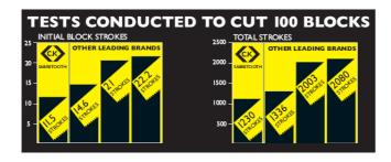
\*1<sup>st</sup> fix saw tested against other leading saws in independent CATRA tests
